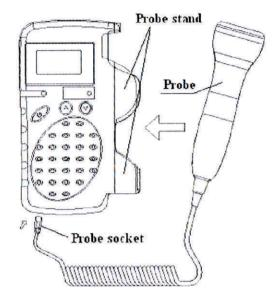
(1) Insert the Probe socket into the socket which is on the main unit.
