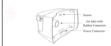
Power Connector: Plug this connector into the power outlet on the BMC RESmart Device.
