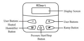
IMPORTANT! In the Setup Menu, the +/- user buttons are used to go to the previous/next question or setting and operate as up and down keys to change the settings, the ramp button is used to confirm the setting change, and the start/stop button will allow you to exit the Setup Menu without saving.
