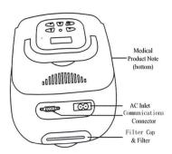
AC Inlet ...... Connect/disconnect the AC power cord here.
